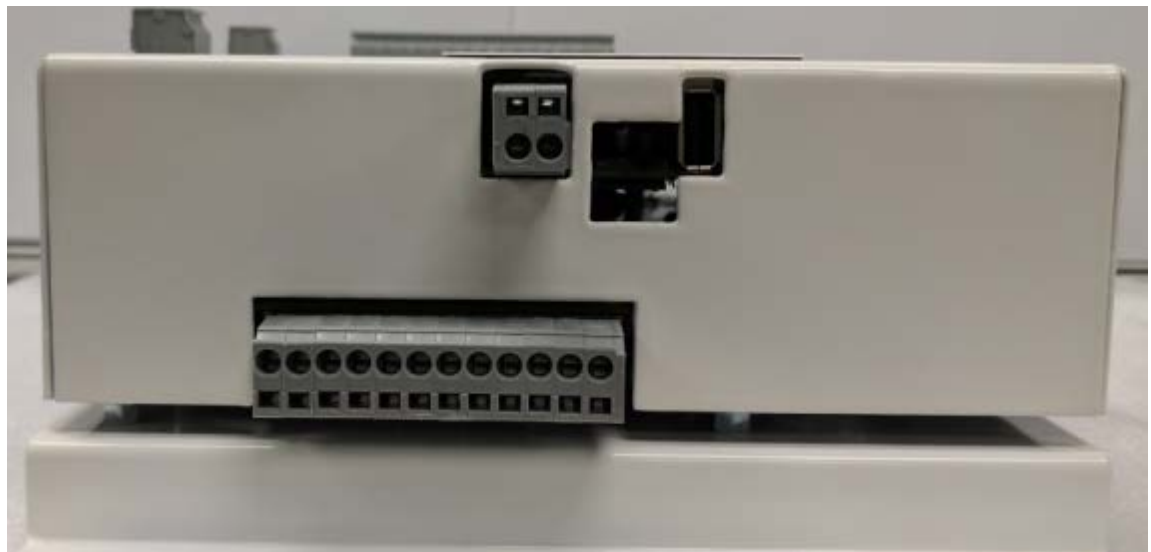
Figure 3. Side of Multiple Cell Monitor
